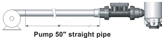
**Note:** Flow Meter Sensor must be mounted in the following orientation with the LED facing up. Ensure all air is purged from the piping and Flow Meter Sensor. All straight length to the Flow Meter Sensor must be 1.00" in diameter.
