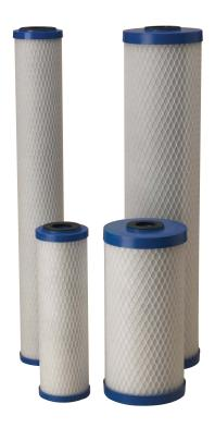
The Pentair<sup>‡</sup> Pentek<sup>‡</sup> EP Series Carbon Block Cartridges are manufactured using a process that yields a cartridge with a nominal 5-micron filtration rating and high dirt-holding capacity. A high porosity design helps prevent the cartridge from plugging before its adsorption capacity is exhausted, maximizing the utilization of the carbon while maintaining low pressure drop.
