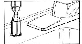
Use the appropriate tool to drill the base material.
