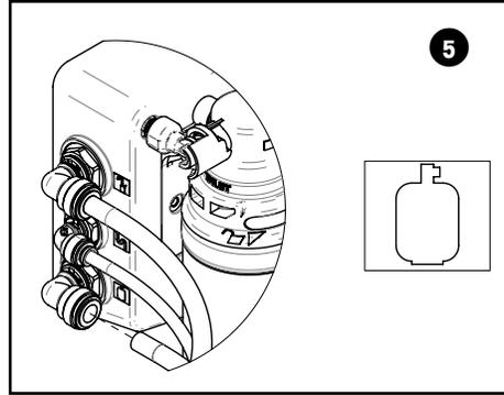
5. Connect the 3/8" OD white product water tube from the tank to the manifold.
