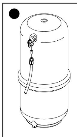
2. Slide compression nut over end of 3/8" white tubing, place the insert in the end of the tube. Connect the white 3/8" tubing to tank using the compression nut.
