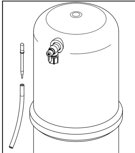
3. Using a clean eye dropper insert 1/2 teaspoon of hydrogen peroxide or common household bleach into the tube.
