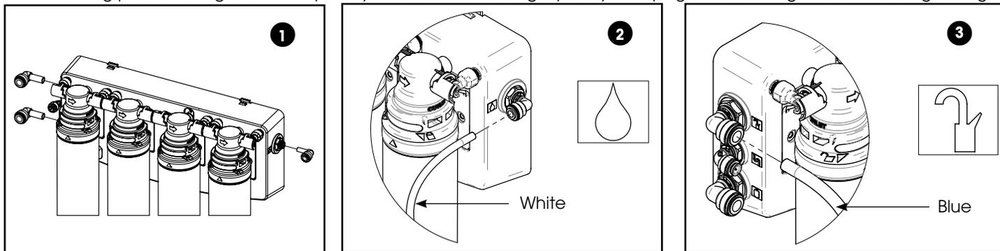
1. Connect quick connect elbows to the three open connection locations on the unit. Firmly push the fittings into place, then pull back lightly to lock them in.
