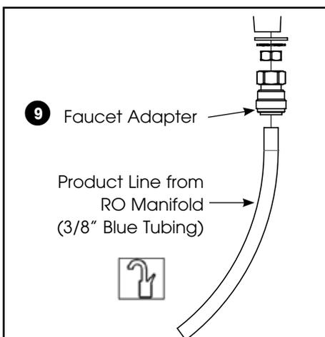
3. Take another length of  $3/8"$  tubing and make sure it has a fresh cut and is free of foreign materials and any scratches on the outside surface. Install the tubing into the push in type fitting at the base of the faucet. Make certain that it is inserted all the way in; once inserted give it a slight pull to make sure it is locked into the fitting. You have now completed the tubing connections.
