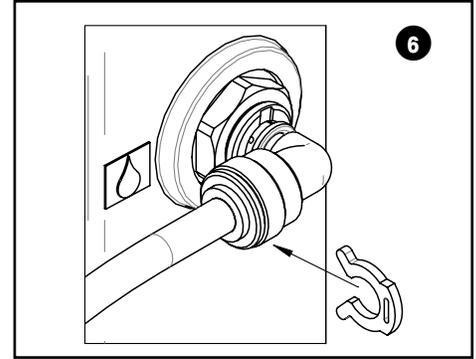
6. Attach locking clips to each white elbow fitting. Do not attach one to the blue flow control. Clips should slide in behind collet on the fittings.
