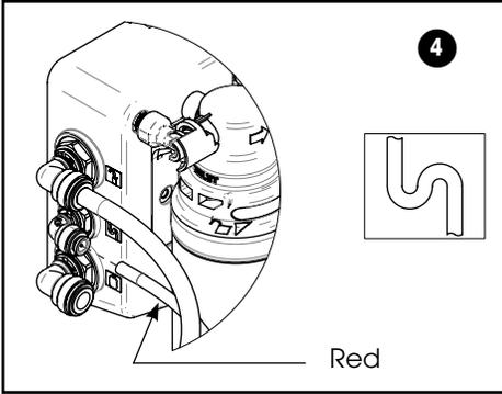
4. Connect the 1/4" OD red tubing from the air gap inlet of the faucet to the concentrate outlet on the RO manifold.
