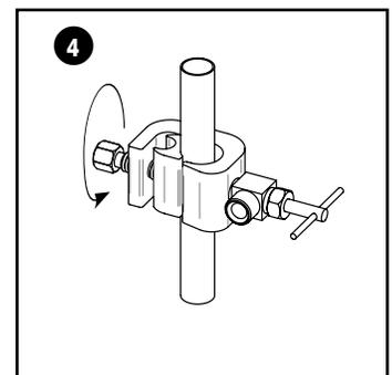
4. Tighten screw firmly so saddle valve is held securely in place. Do not crush tube.
