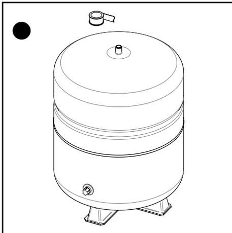
1. Apply teflon (PTFE) tape to threaded fitting at top of tank. Wrap tape around clockwise 3 to 6 times for a good seal.
