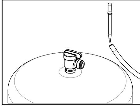
3. Using a clean eye dropper insert 1/2 teaspoon of hydrogen peroxide or common household bleach into the tube.
